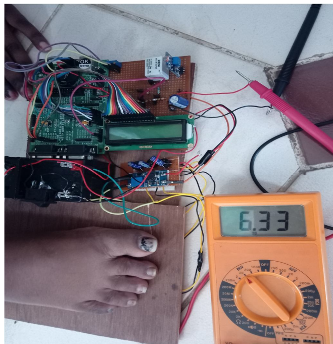
Fig 7 Implemented system to observe the capacitor voltage generated for various trials of pressure applied.
