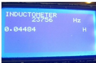
Fig.14 Result of a tested inductor
