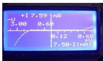
Fig.11 I-V characteristics curve of a tested Zener diode
