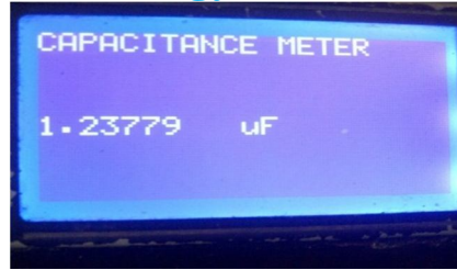
Fig.15 Result of a tested capacitor
