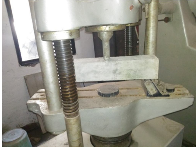
Fig .6 Flexural strength test on beam
