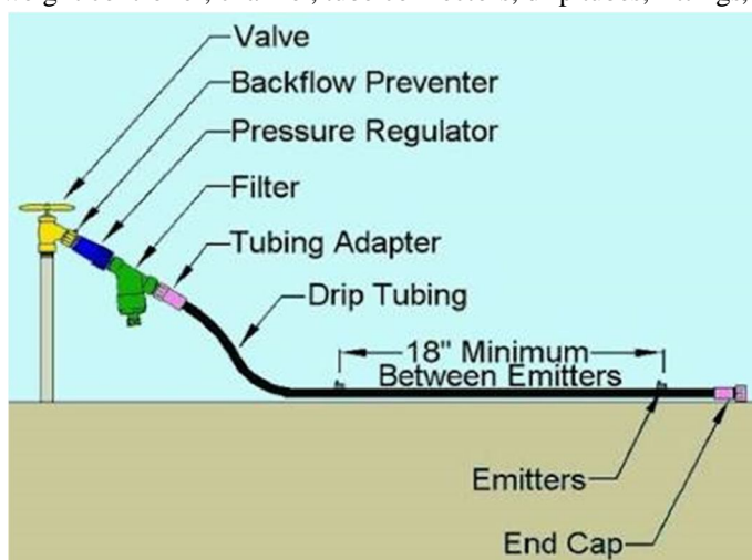
Fig. 3. Drip irrigation system
