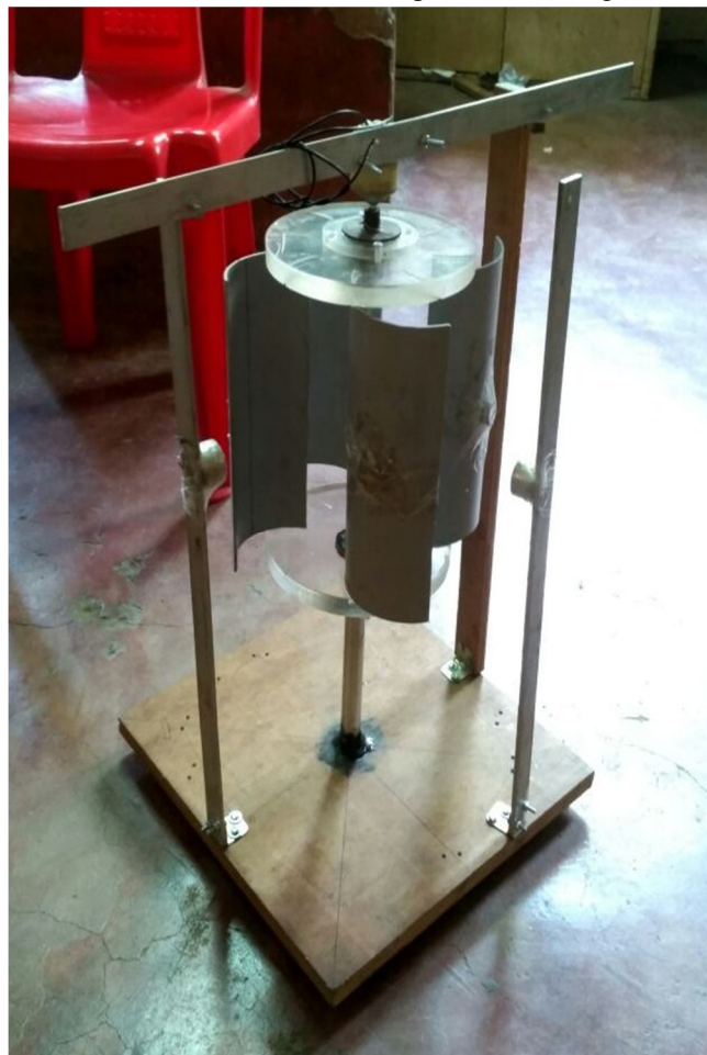
Fig.7: Experimental Setup of VAWT to generate free power
