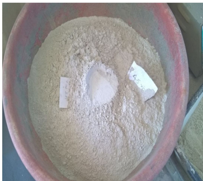
Fig 1: Ground Granulated Blast Furnace Slag
