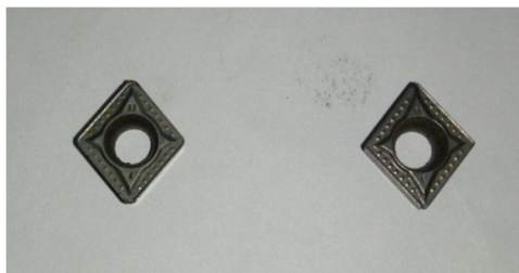
Fig 2: Alumina coated tungsten carbide tool
