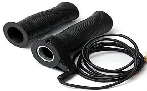
Fig 4: Throttle of E- Bicycle
