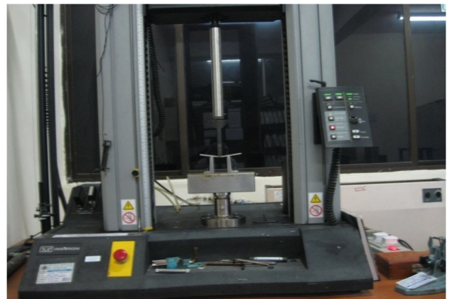
Fig 4: Specimen Under Flexural loading
