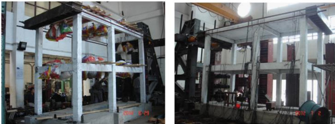
Fig. 2.8: The loading setup.
