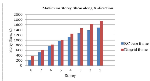
Fig 7. Maximum storey Shear of C-shaped RC frame & diagrid frame models in Zone-V at each floor level subjected to EQX
