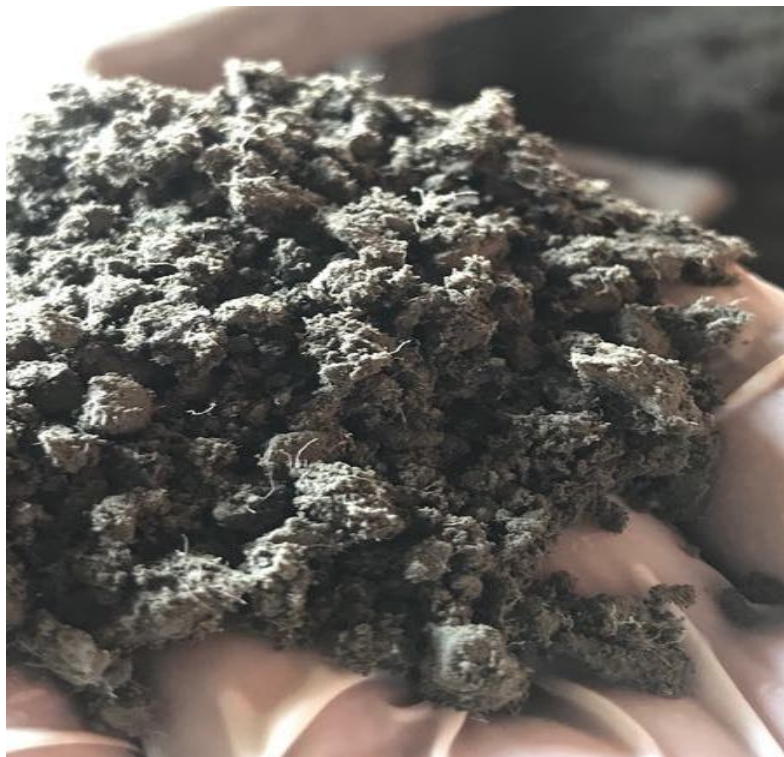
Figure 6: Cellulose Acetate fibres mixed with the constituent materials of concrete
