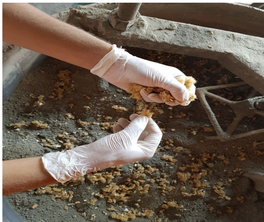
Figure 5: Mixing the constituent materials of concrete with grinded cigarette butts
