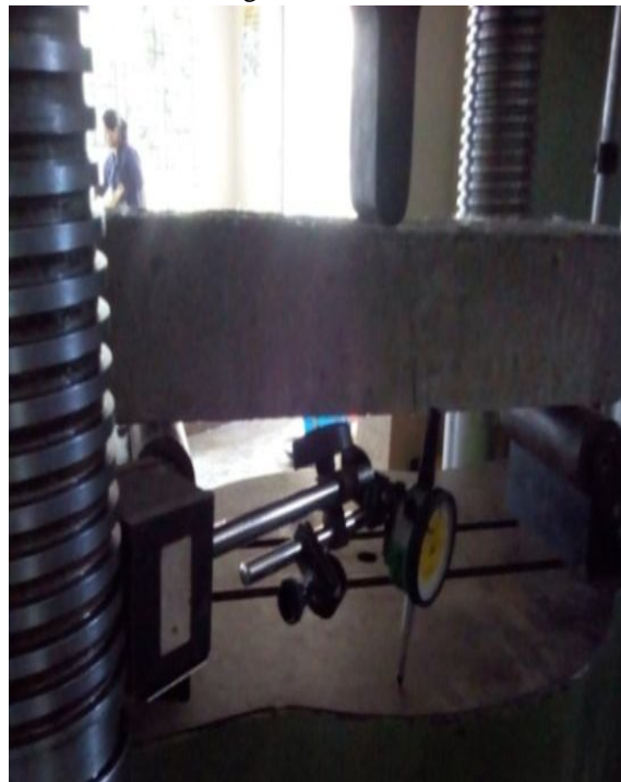
Fig 4 Fracture test loading arrangement
