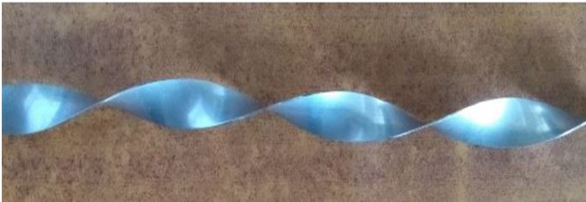
Fig. 3 Plain twisted tape
