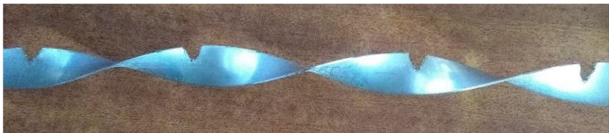
Fig. 4 Notched twisted tape
