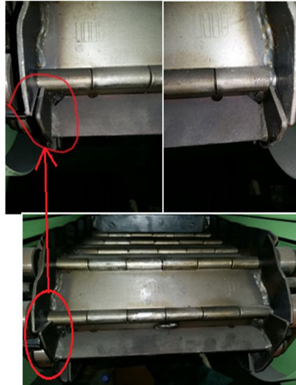
Fig. 10 Side Wing Gap
