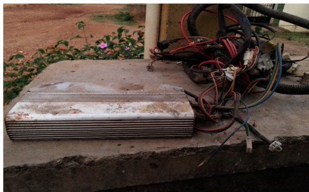
Fig 3: Three Phase Controller
