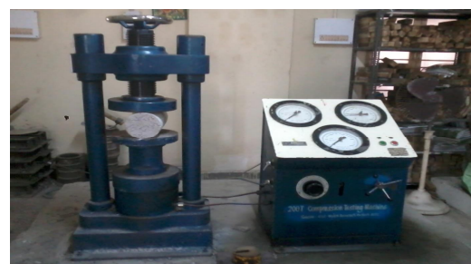
Split tensile testing
