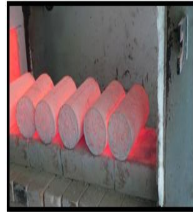
Bogie hearth furnace testing cylinders
