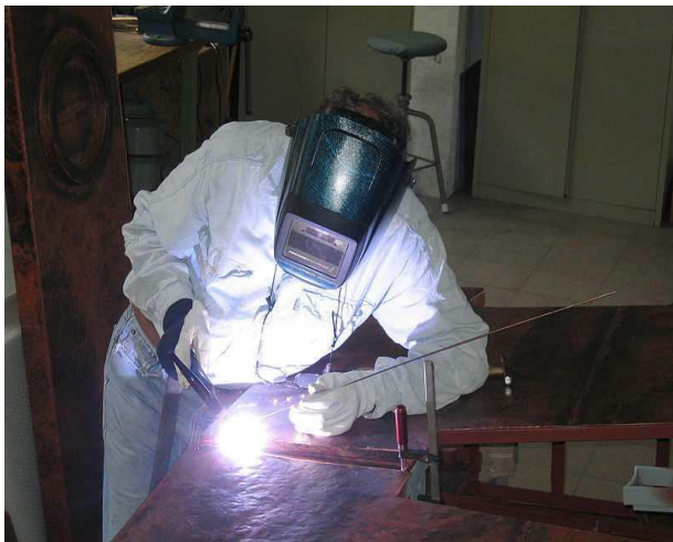
TIG welding process
