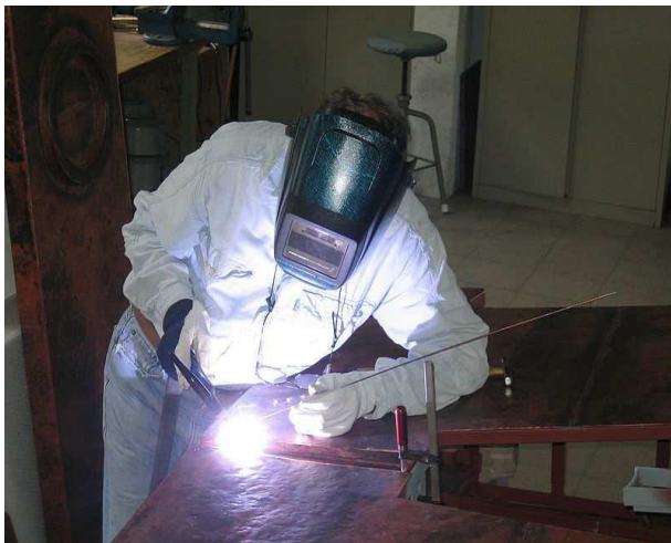
TIG welding process
