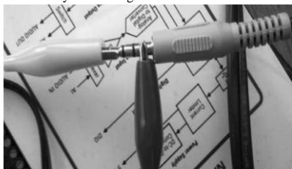
Fig 17. 3.5mm male-male jack connected to the sound card
