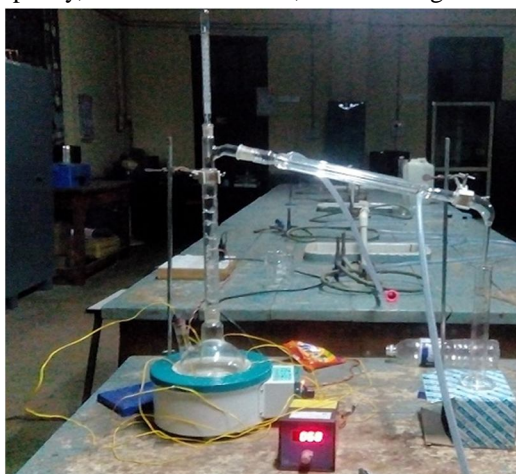
Fig. 1 Fractional distillation set-up
