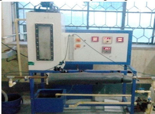
Fig.1 Tubular Heat Exchanger set up
