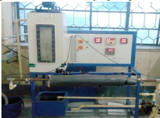
Fig.1 Tubular Heat Exchanger set up
