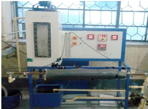
Fig.1 Tubular Heat Exchanger set up
