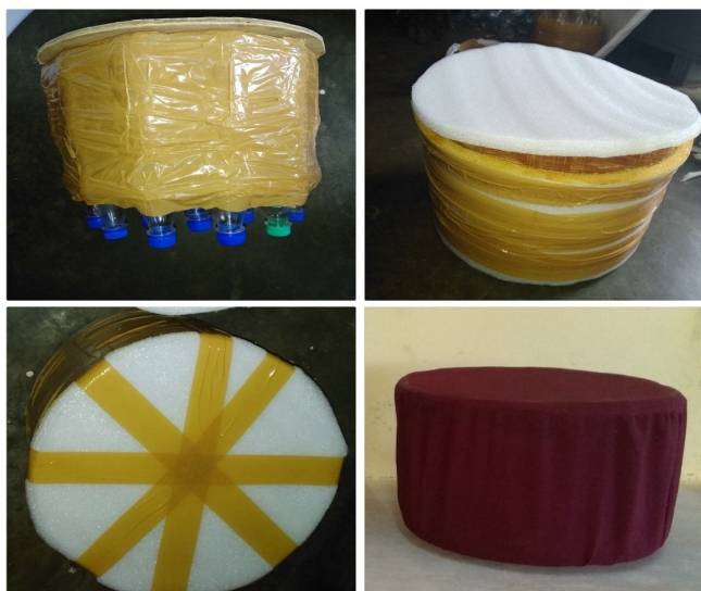
Fig. 2: Adding thermocol to side surface of stool which will provide strength and exact shape to the body, adding tape so that glue may work properly, and in final step covering with cloth or other plastic painting as per availability.
