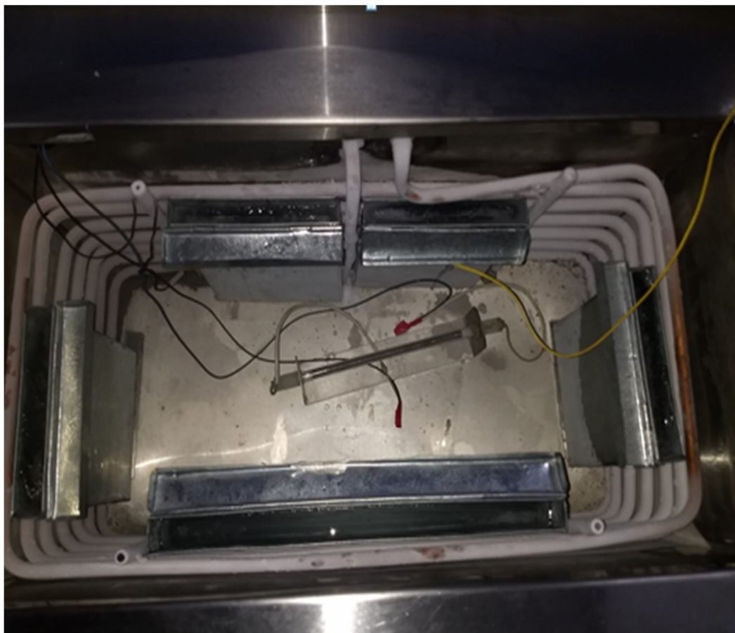
Fig.2 Low side evaporator cabin with PCM
