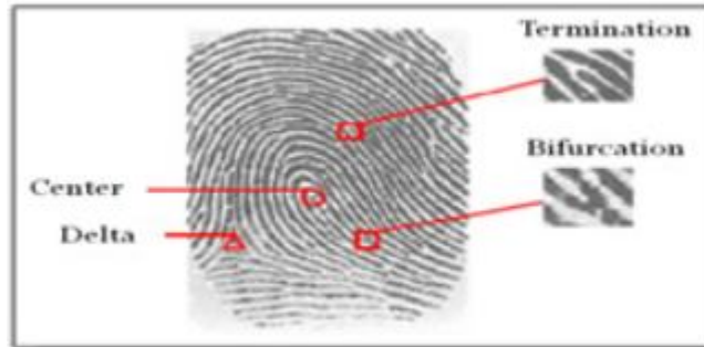
Fig. 2. Local and Global singular points in a fingerprint
