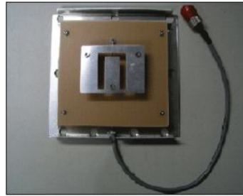
Fig.2. practical U-slot patch antenna
