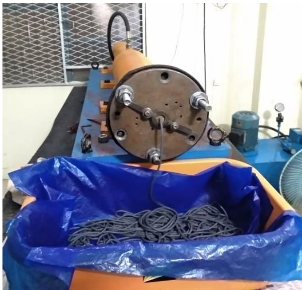
Figure 4.5: Abrasive media extruded through specimen
