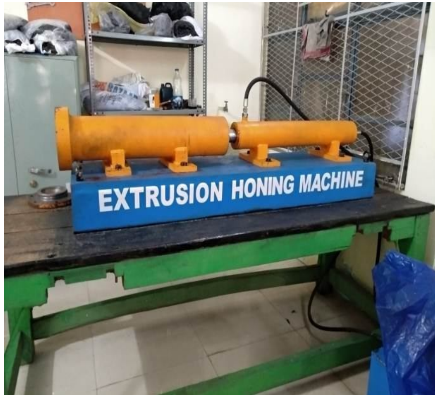
Figure 4.1 Extrusion Honing Machine
