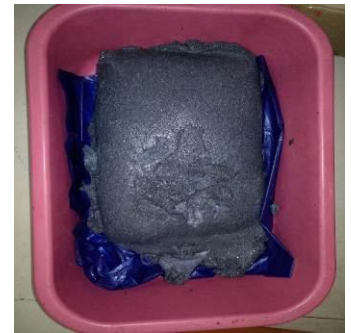
Figure 4.4: Silicon polymer with abrasive
