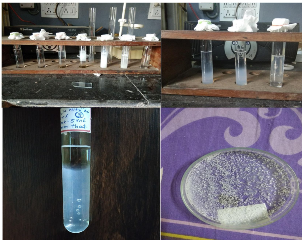
Fig.3 Gel Method and Grown Crystals
