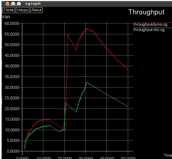
Figure 14: Graph output showing Throughput vs time
