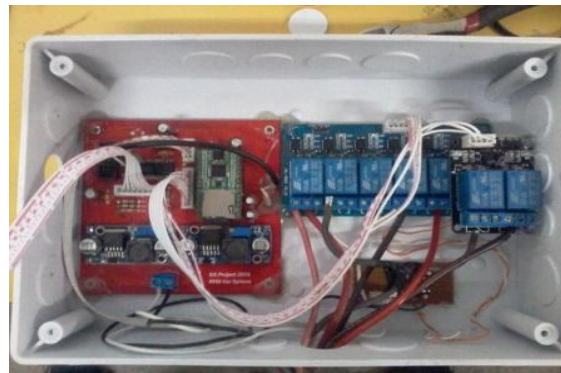
Fig. 6 The Control System Circuit.
