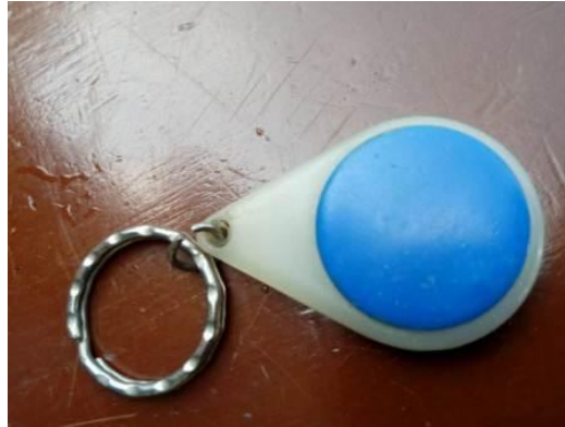
Fig. 5 RFID Mifare Tag as a Key holder
