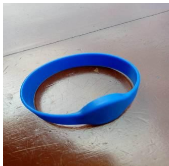
Fig. 4 RFID Mifare Tag as a Bangle
