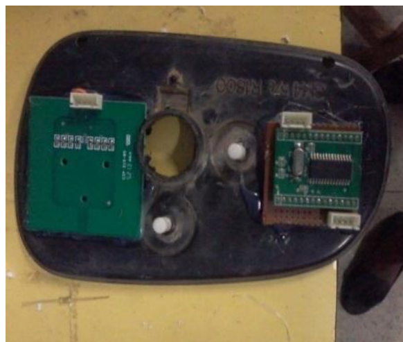
Fig. 20 MIFARE reader and Antenna attached to Side Mirror
