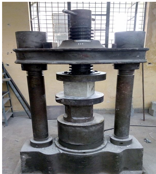
Fig: 4.1 Cube Compressive Strength Test
