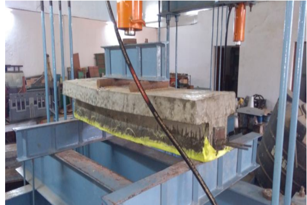
Fig 6:- Deflected shape of Post Tensioned Beam
