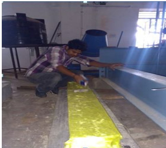
Fig 4: Application of Epoxy and Aramid fibre
