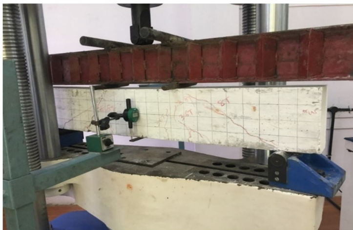
Fig 10: Beam specimen for M30 grade
