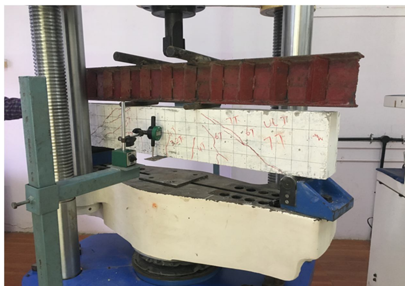
Fig 11: Beam specimen for M25 grade
