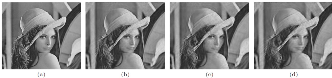
Figure 7: (a) Original image, 256 by 256, 8bits/pixel,with MSE = 0, PSNR = 1, (b) Restored image of noise var.0.04,(c)Restored image of noise var. 0.06, (d) Restored image of noise var.0.08
