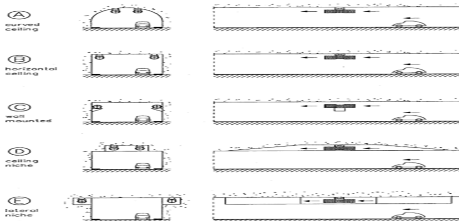
Typical Jet Fan Installations in road Tunnel
