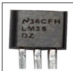
Fig: 6 LM 35 Temperature Sensor
