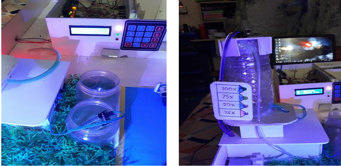
Fig. 8. Reading soil moisture in the garden and IoT based water Tank
