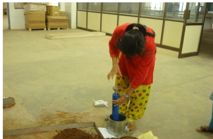
Fig 11. Standard Proctor Test
