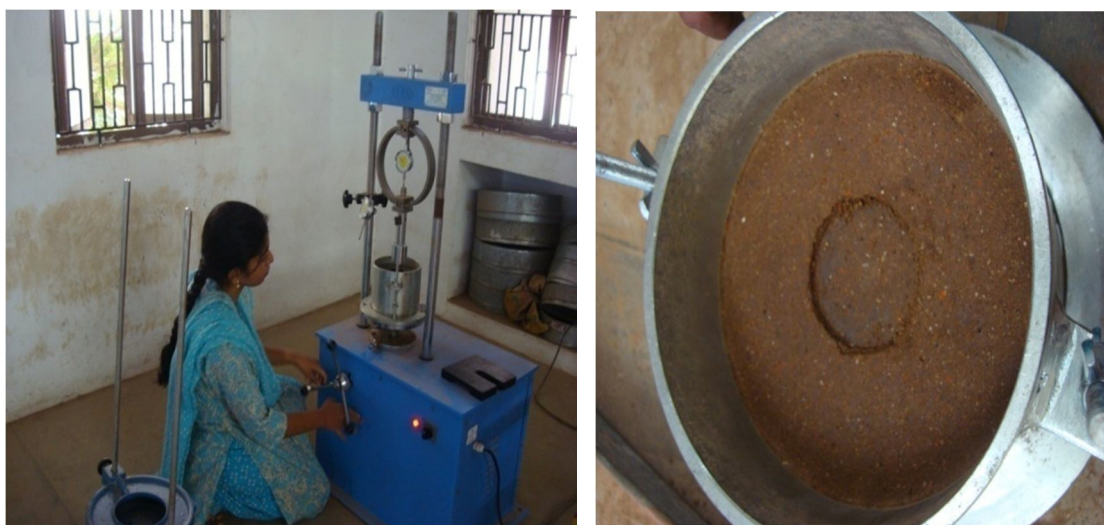
Fig 15. CBR Test of Soil Sample
