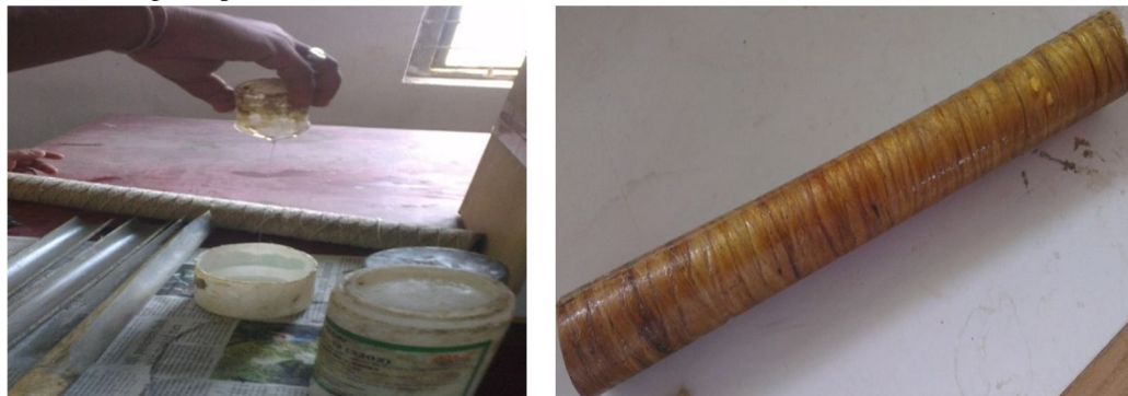
Fig 4: Preparation of composite pipes
