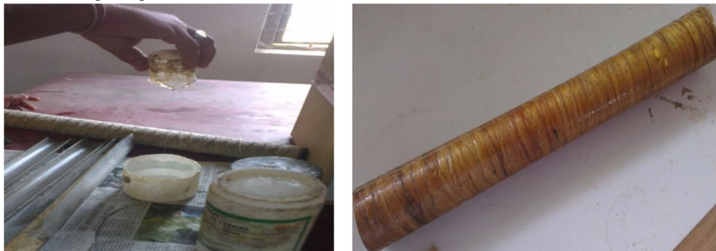
Fig 4: Preparation of composite pipes
