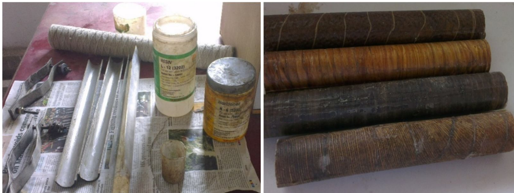
Fig 3: Preparation of composite pipes
