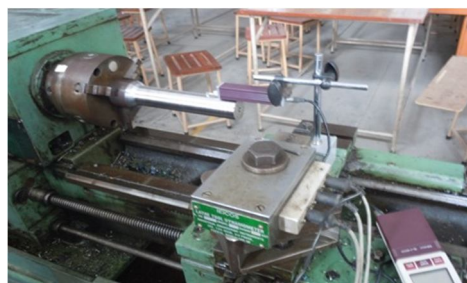
Fig. 2 Measurement of surface roughness
