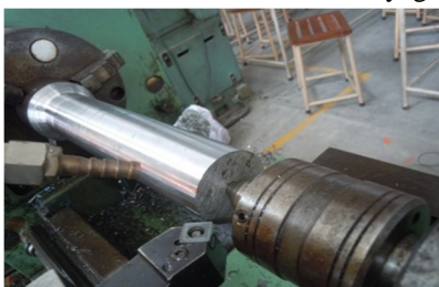
Fig. 1 Coolants used at tip of the tool
