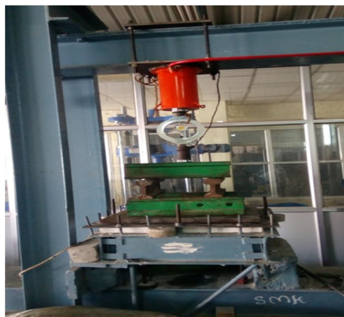
Figure 6.2: Testing of slab for flexural strength
