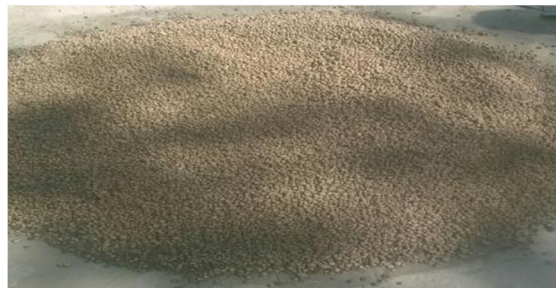
Figure 3.3.3 Sintered fly ash aggregate
