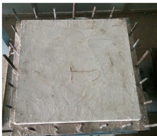
Figure 6.1: Arrangement of slab on simply supported condition
