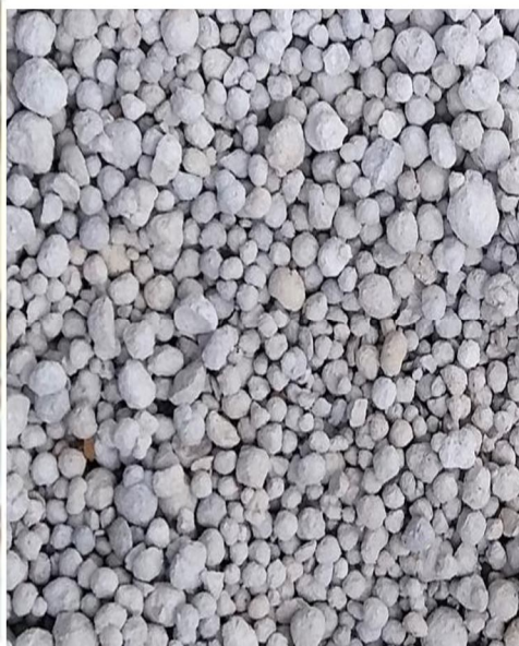
Figure 3.3.2: Silica fume aggregate
