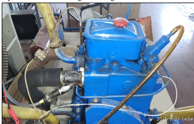
Fig.1: Intake Port Injection system for DME
