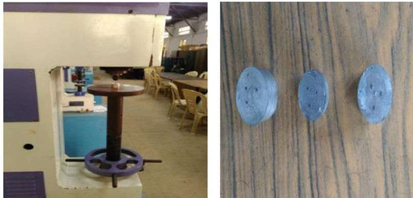
Figure 3 Brinell hardness Tested Specimens
