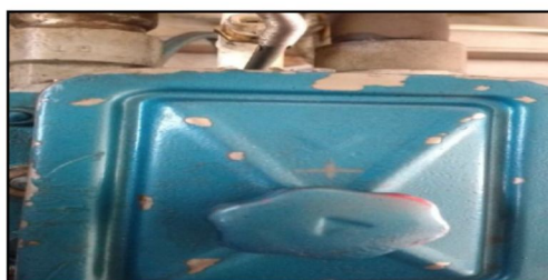
Figure : Location of vibration measurements in linear(x) and Lateral (y) directions
