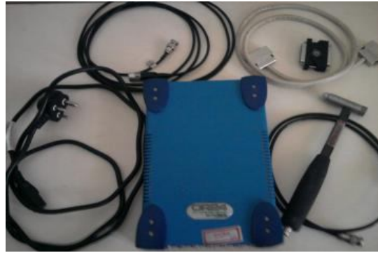
Fig 11: Fast Fourier Transform analyser with accelerometer
