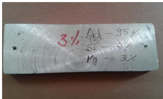
Fig 3: 95% Aluminium + 2% Silicon + 3% Magnesium
