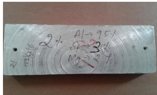
Fig 2: 95% Aluminium + 3% Silicon + 2% Magnesium
