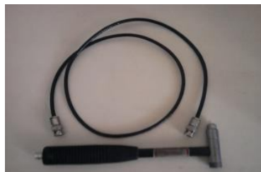
Fig 9: Hammer will be instrumented with a force transducer
