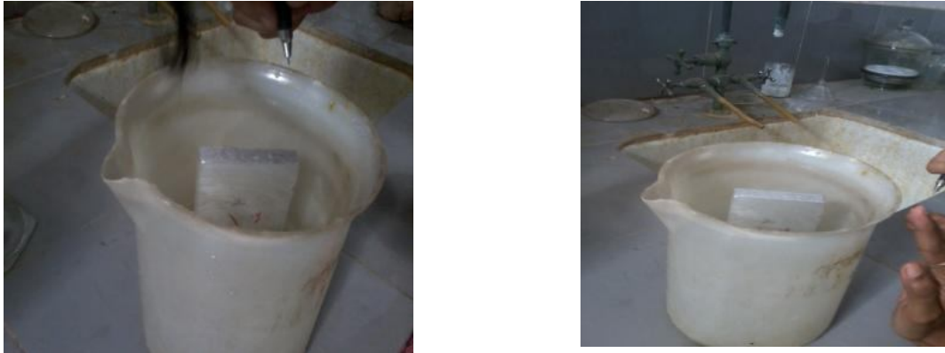
Fig 7: Shows Water Displacement to Measure Volume
