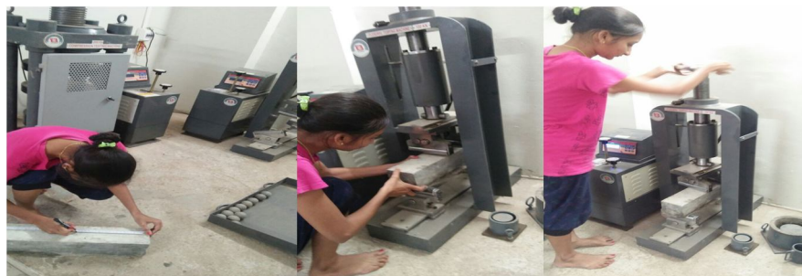
Flexural Strength Test Results At 28 Days (Fly Ash As Partial Replacement Of Cement)
