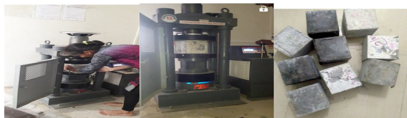
Compressive Strength test results at 28 days ( FLY ASH as partial replacement of cement)
