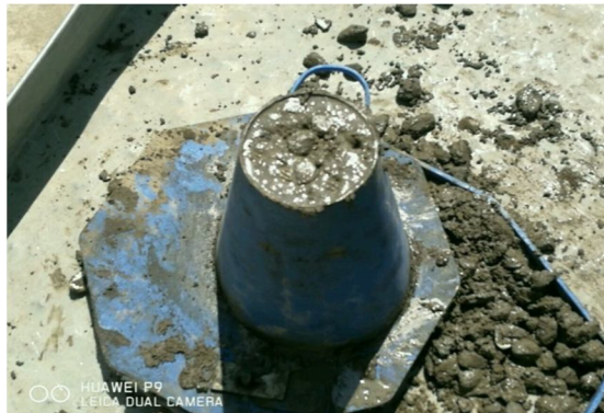
Fig 4.1 Slump Cone Test
