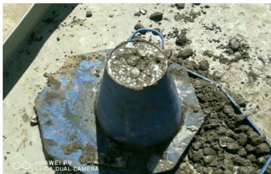
Fig 4.1 Slump Cone Test
