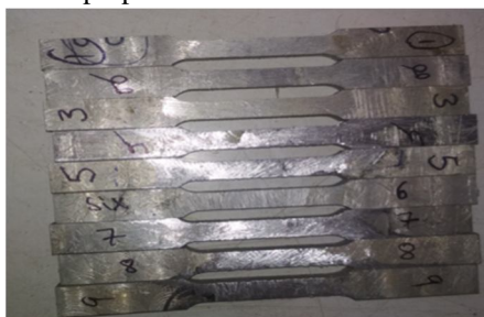
Figure 8: Before test specimen
