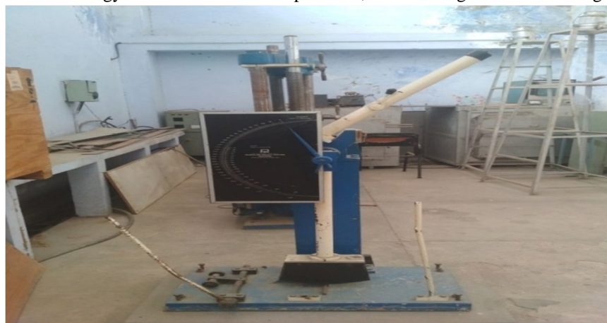
Figure 10: Impact Testing Machine at Metallurgy Lab, SLIET Longowa
