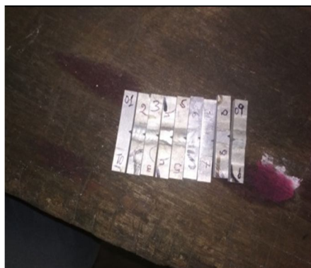
Figure 11: Impact test specimen before test
