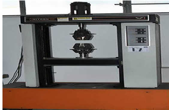
Fig. 8 UTM setup for Tensile test
