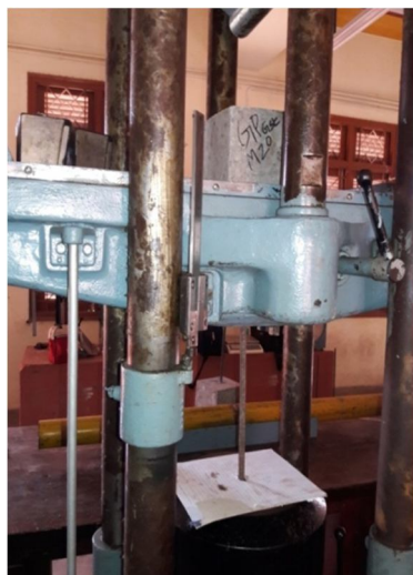
Figure VIII Pull Out Test Set up (RWGCA Specimen)
