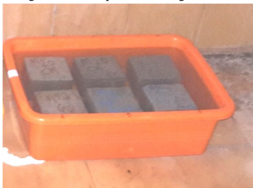
Figure V Specimens Immersed in MgSO 4 with Na 2 SO 4 Solution
