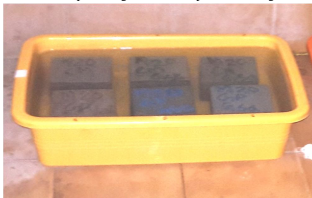
Figure IV Specimens Immersed in H 2 SO 4 Solution
