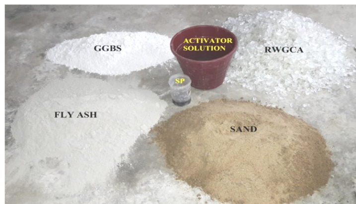
Figure III Materials used for RWGCA Geopolymer Concrete
