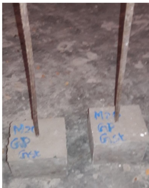
Figure VII RWGCA Specimens Before Testing
